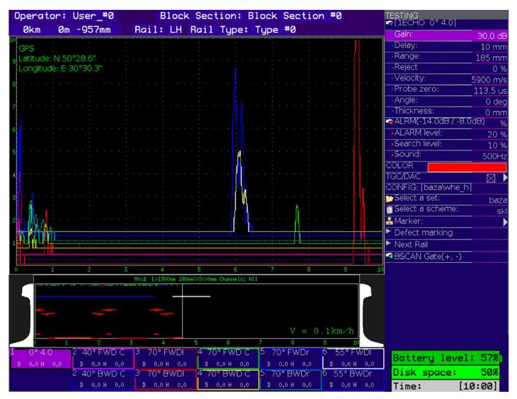
Date/Time:08.28.2023:07.02 SRT serial number:Sr.No. - 2308337 Operator:User\_#0 Division:Division #0 Block Section:Block Section #0 Line:Up Current Position:0Km 0m Start Position:0Km 0m Rail:RH Rolling mark:5236 Location defect:
