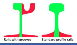
The rail flaw detector deploys a unique scanning scheme that allows you to test the entire section of the rail, except for the foot flanges and the checkrail, using the pulse echo, echo-shadow and echo-image methods.
